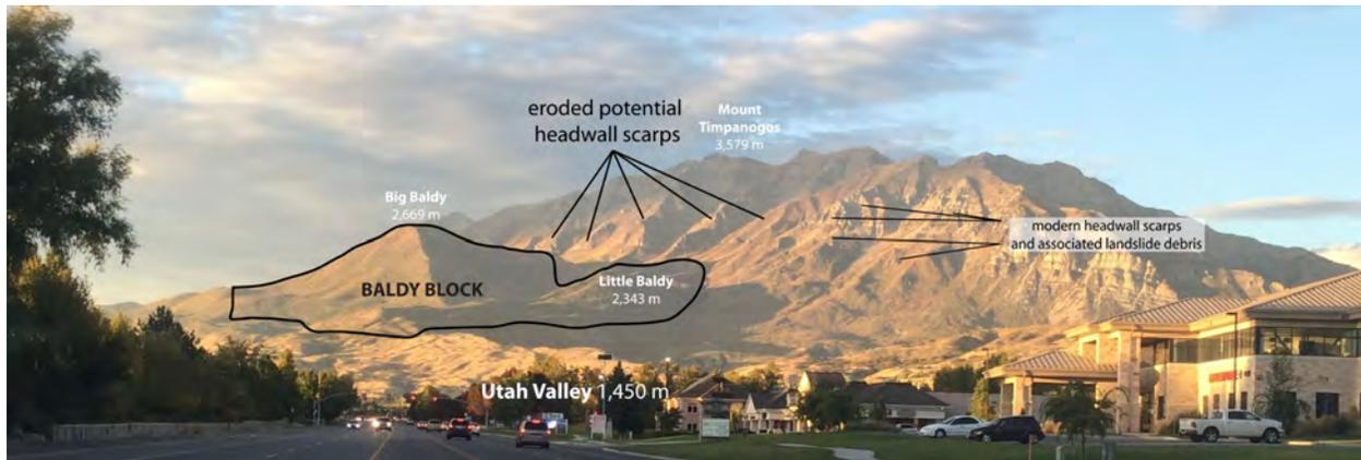
**Figure 8.** Potential remnants of the headwall scarp of the Baldy slide on Mount Timpanogos. Directly above the Baldy block are highly eroded possible landslide scarps (as indicated by the pyramid-shaped group of lines on the left), adjacent to modern scarps caused by more recent slope failures (indicated by the horizontal lines on the right).
