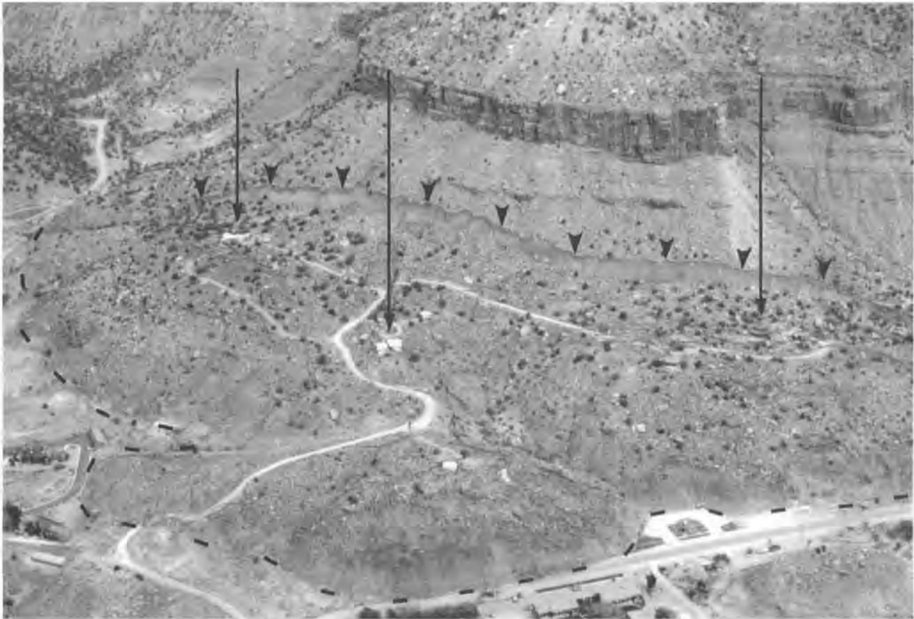
Figure 13. Aerial view of the Springdale landslide (from Black et al., 1995). Utah Highway 9 is at the bottom; short arrows show the main scarp of the landslide, long arrows indicate three houses damaged, medium arrow locates an abandoned water tank, and dashed line outlines landslide toe.
