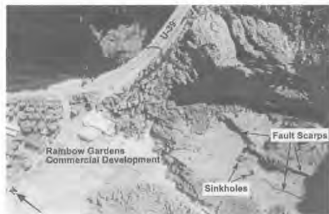
Figure 23. Sinkholes along a normal fault crossing the frontage trough, Ogden River landslide complex.
