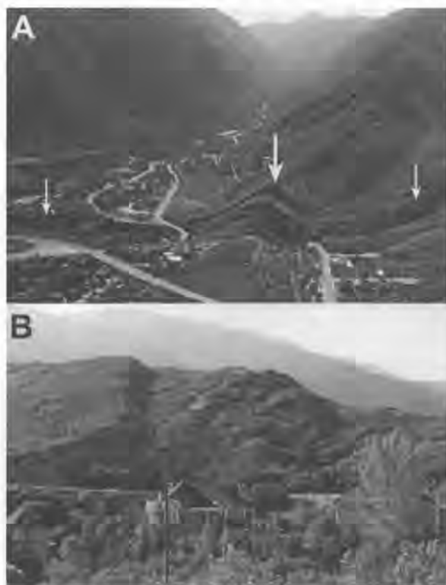
Figure 3. Wasatch fault zone at the mouth of Little Cottonwood Canyon. A. Aerial view, looking east, of fault scarps (arrows) cutting upper Pleistocene moraine and alluvial deposits. B. South view of fault scarps (in shadow) cutting Bells Canyon moraine (large arrow on Fig. 3A). Residential development in foreground occupies a graben along the fault zone.
