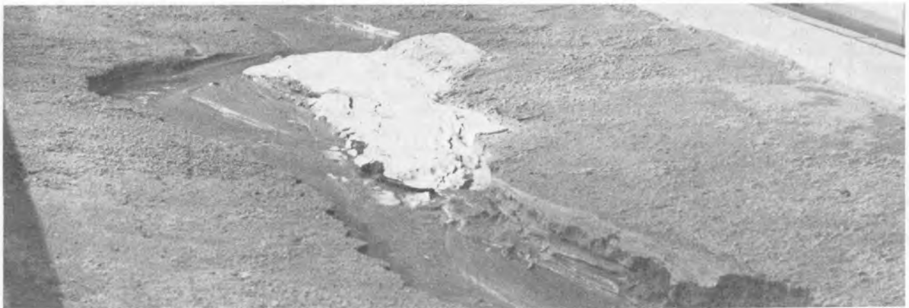
FIGURE 10.—As the stream reached the level of the original gradient, quasi-equilibrium was approached. The "basalt" was left as an isolated ridge along one margin of the new channel.
