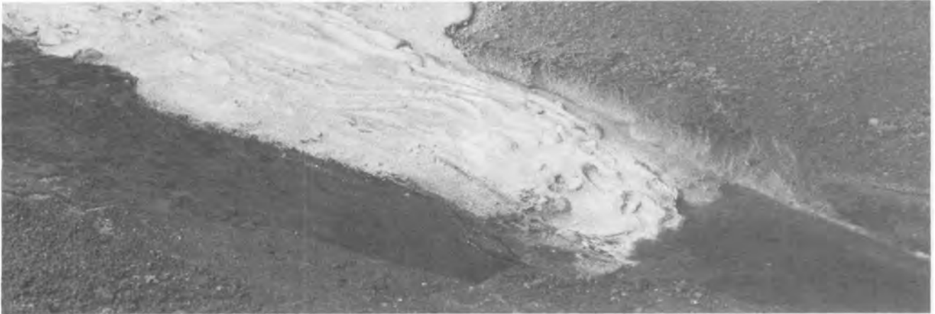
FIGURE 6. —Water overflowed along the margin of the "basalt" dam and reentered the original channel at the end of the flow. Headward erosion progressed very rapidly along this margin, as can be seen by the simulated rapid falls. Deposition also occurred at the front of the cement-filled channel in order to build up the gradient to a profile that developed a state of equilibrium.
