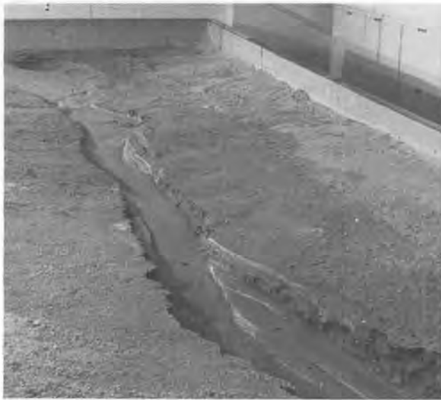
FIGURE 3.—The stream table was operated for a period of time, and a stream profile developed that was in a state of quasi-equilibrium.
