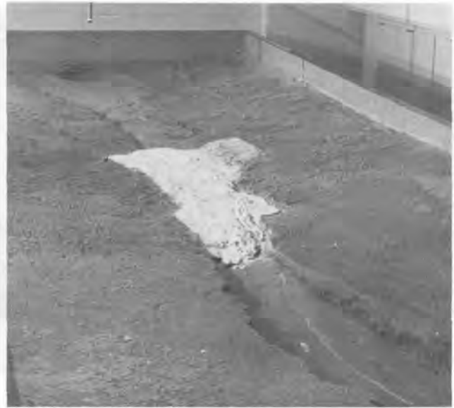
FIGURE 4.—Cement was mixed into a viscous fluid, poured into the stream channel, and allowed to harden simulating a basalt flow and cone. The cement represented the more resistant basalt, and the sand represented the less resistant sedimentary rocks.
