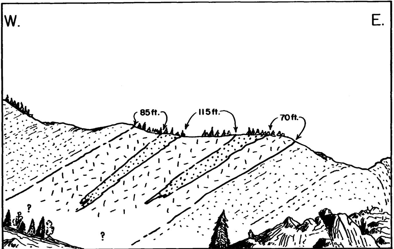
Fig. 2 Field sketch showing details of sill I-F, North Willow Canyon.
